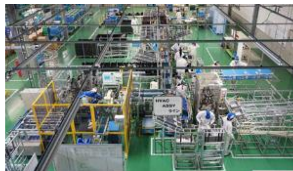
Production line for air-con units for mini vehicles (Suzuka Plant, Japan)
