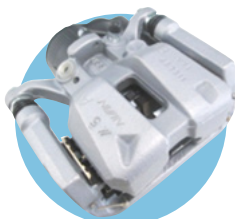
Rear caliper (electronic parking brake)
